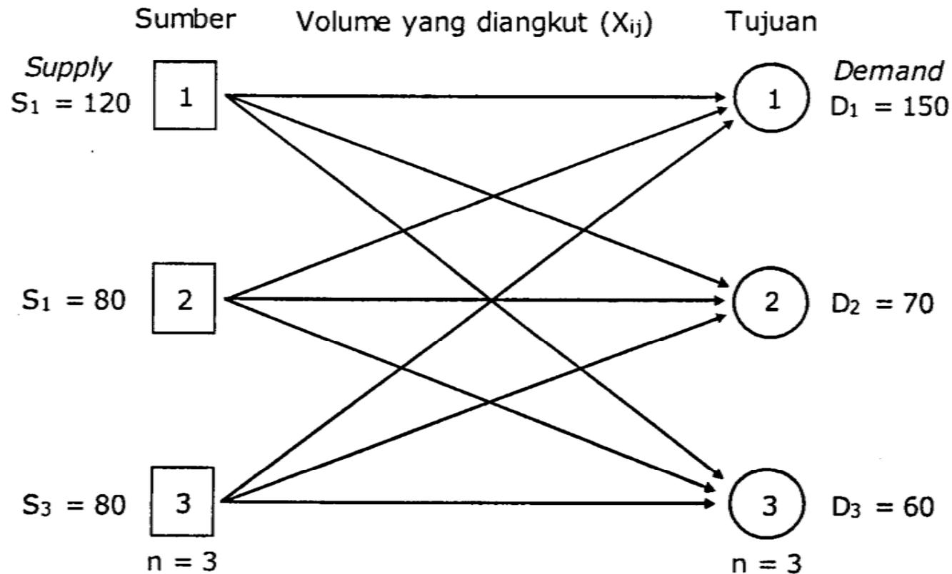
Minimumkan  $Z = 8X_{11} + 5X_{12} + 6X_{13} + 15X_{21} + 10X_{22} + 12X_{23} + 3X_{31} + 9X_{32} + 10X_{33}$
