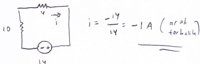
3. Find the Norton equivalent of the circuit to the left of terminal a-b, and use the result to find  $i$ .
