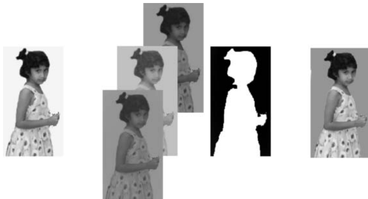
Figure 14-13 Representation of arbitrary shaped VOPs. The left image shows a VOP of arbitrary shape. The central set of images shows an explicit representation of the VOP shape, which is given by the alpha channel of the VOP. The image on the right shows an implicit representation, where green chroma suggests background.
