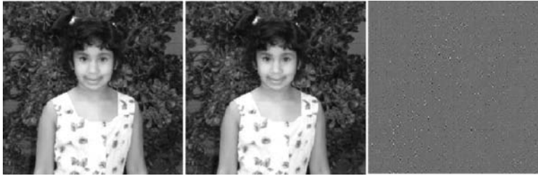
Figure 13-7 Original image, heavy watermarked image using adapting relationships between DCT coefficients and W(x,y) = I(x,y) - I_w(x,y)
