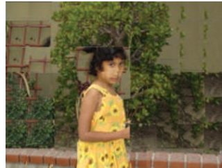
Reconstructed frame n+1 by macroblock prediction
