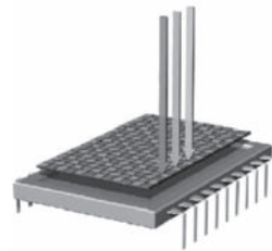
Bayer mosaic pattern overlaid on a CCD chip
