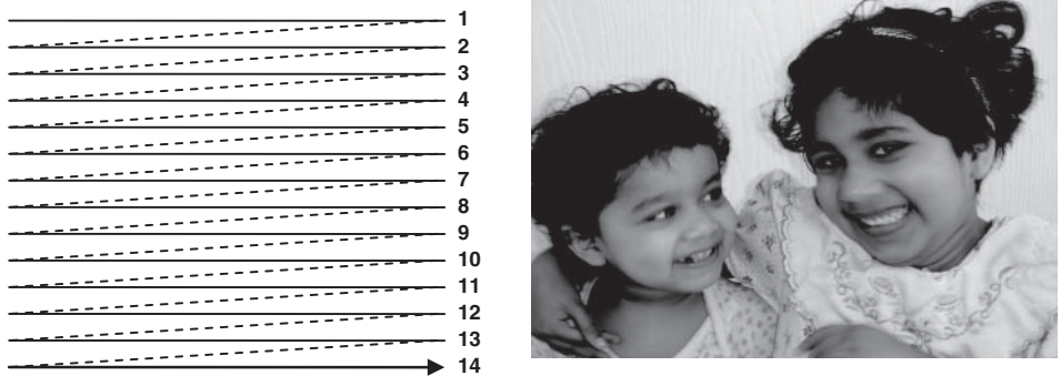
Figure 3-11 Progressive scanning. All the scan lines are drawn in succession, unlike in the interlaced case.
