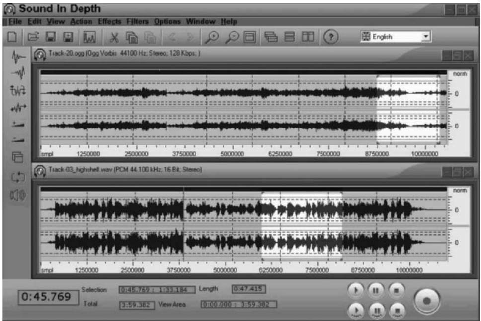
Figure 5-7 An audio-editing tool— In Depth . Shown are highlighted sections of stereo audio samples in the sound data file. These samples can be edited out, filtered, attenuated, and so on depending on the desired effect.
