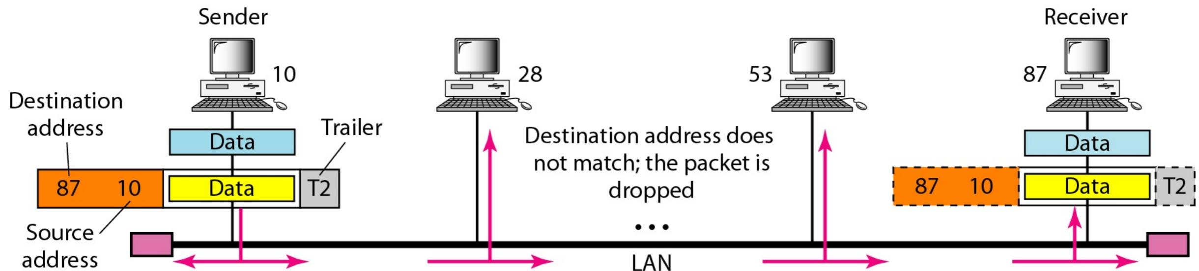
In Figure, a node with physical address 10 sends a frame to a node with physical address 87. The two nodes are connected by a link (bus topology LAN). As the figure shows, the computer with physical address 10 is the sender, and the computer with physical address 87 is the receiver.
