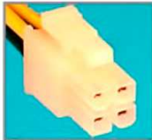
ATX12V Connector 4 Pin
