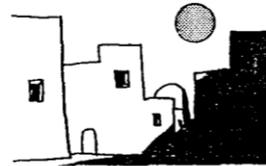
In hot dry areas thick walls keep out the heat by day, light colours reflect the sun's rays and small windows minimise glare.
