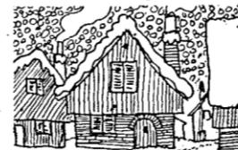
Where it is cold and wet thick dark walls of brick or wood both keep out the cold and store heat. As the sky is less bright, large windows are needed.
