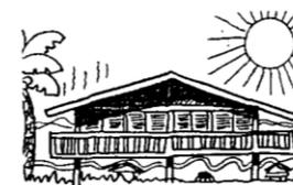
In tropical regions where it is hot and humid walls become open screens to let air pass through but keep out the heat. Verandahs and roof overhangs provide shaded outdoor "rooms".
