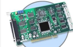
**OME-PCI-1000 Series Data Acquisition Plug-in Boards**
