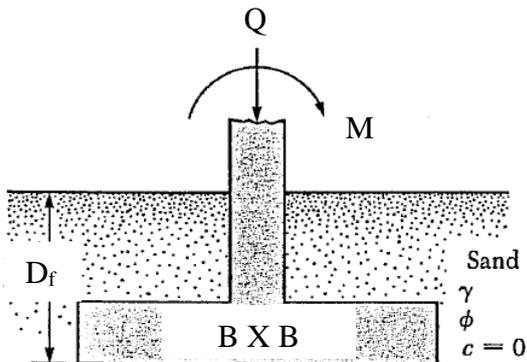
A square foundation is shown in figure. It is subjected to a load  $Q$  and a moment  $M$ . Using a factor safety of  $SF = 3$ , determine the size of footing ( $B$ ) if:
