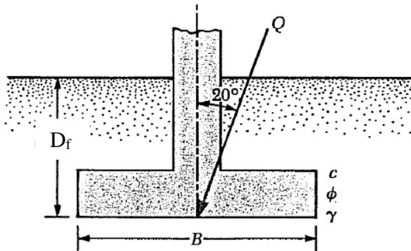
A square column foundation has to carry a gross allowable total load of  $Q$ . The depth of the foundation is  $D_f$ . The load is inclined at an angle of  $20^\circ$  to the vertical. Determine the allowable gross load with a factor safety of 3 using Meyerhof's Bearing Capacity Equation with shape, depth and inclination factors from:
