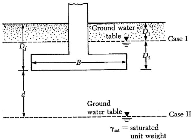
A square foundation is  $B \times B$  m in plan. The soil supporting the foundation has a friction angle of  $\phi$  and  $c$ . The unit weight of soil  $\gamma$  and saturated unit weight of soil  $\gamma_{sat}$ . Assume that the depth of foundation is  $D_f$  and that general shear failure occurs in the soil.
