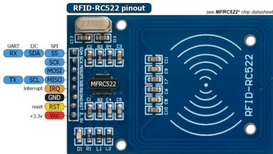
Gambar 2. RFID RC522 Pinout
