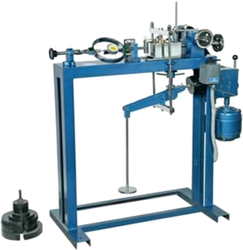
Alat geser Langsung (Direct Shear)
