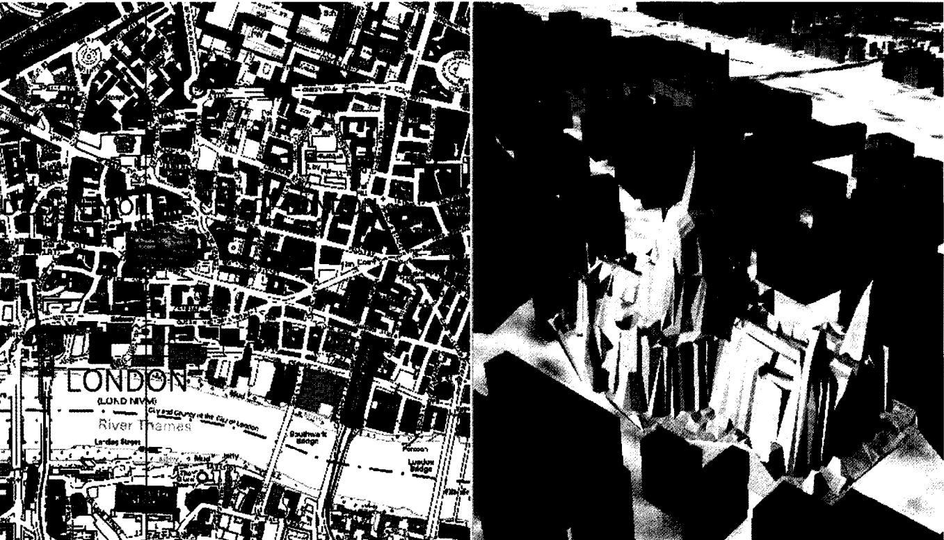
FIGURE 6: A GIS 3D block model of St Paul's district in the city of London with height data from LIDAR data
