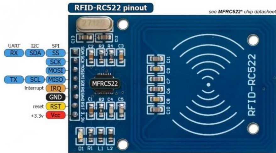
Gambar 2. RFID RC522 Pinout
